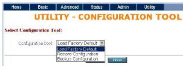
named backup. Press Finish. The router will automatically backup the configuration.
